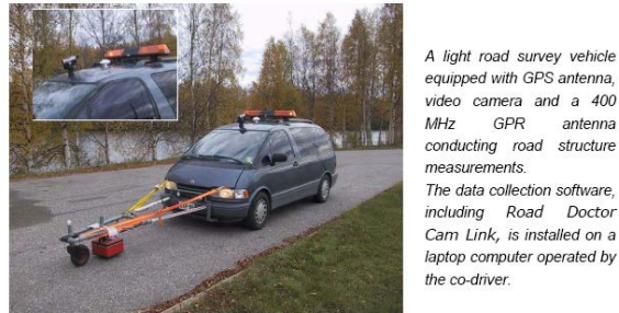
Figure 13. A vehicle system with the GPR and GPS is used for continuous Roadway surveys 71
