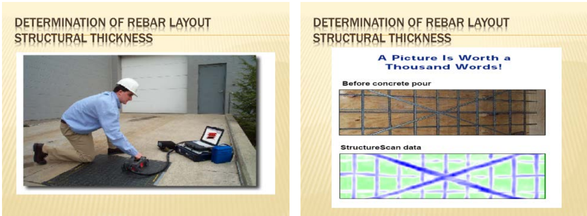
Figure 15. The scanning and actual layout vs the scanned layout is shown in the above pictures from Mala Geosciences
